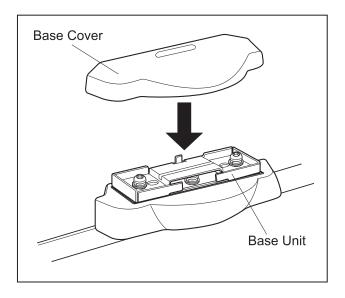
After removing the stay and the bar, leaving only the base unit on the vehicle, apply the base cover to the base unit.
