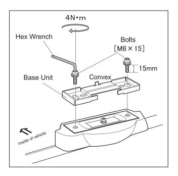
Place the base unit on the installed cushion base/base bracket. Then using the Hex wrench (included), tighten while alternating between the right and left bolts (short) [M6x15] (supplied with the carrier) until the bolts are firmly tightened.
