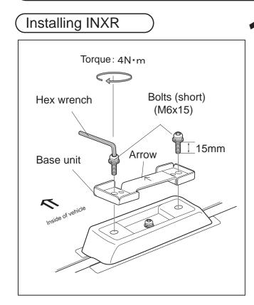
Place the base unit on the installed cushion base/base bracket, and using the Hex wrench, tighten alternately the right and left bolts (short) [M6 x 15] supplied with the carrier until the bolts are firmly tightened. The base unit must be placed as the arrow on the unit faces toward the vehicle center.
