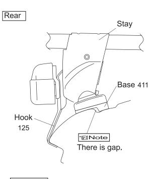
When knob is tightened, base moves slightly outward to the position illustrated above.
