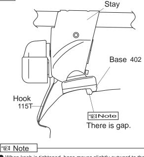
When knob is tightened, base moves slightly outward to the position illustrated above.
