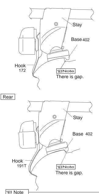
When knob is tightened, base moves slightly outward to the position illustrated above.
