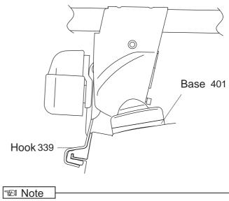
When knob is tightened, base moves slightly outward to the position illustrated above.
