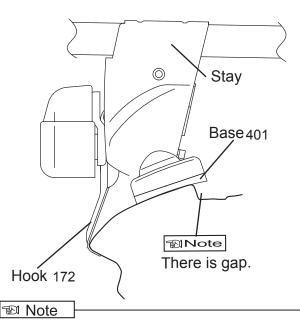
When knob is tightened, base moves slightly outward to the position illustrated above.
