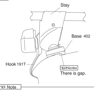
When knob is tightened, base moves slightly outward to the position illustrated above.
