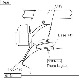
When knob is tightened, base moves slightly outward to the position illustrated above.
