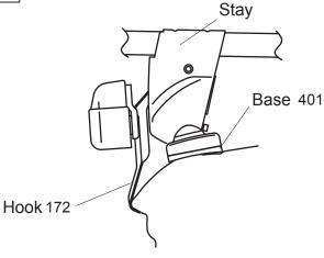
When knob is tightened, base moves slightly outward to the position
