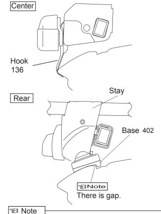
When knob is tightened, base moves slightly outward to the position illustrated above.
