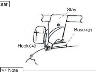
When knob is tightened, base moves slightly outward to the position illustrated above.
