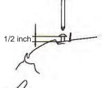
Slot the groove of hook into space between head of screw and roof.
