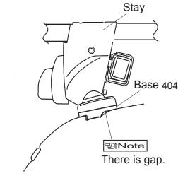
Hook installation position for center hook is the same as front carrier.
