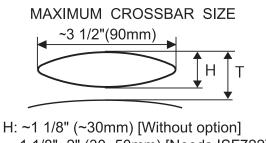
1 1/8"~2" (30~50mm) [Needs ISF722] T: Distance to Roof : Min2 3/8" (60mm)
