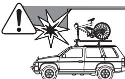
Check the height of the loaded bicycle before driving the vehicle. Do not enter a parking lot or tunnel whose ceiling is lower than the loaded bicycle height.
