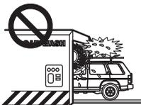
Remove the carrier before using an automatic car wash. Should the car mistakenly be washed by an automatic car wash with the carrier attached, be sure to inspect the carrier.
