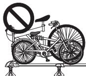
Do not load a bicycle that does not conform with this product. Do not load 2 or more bicycles on one attachment.
