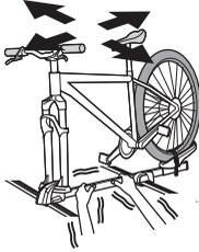
Shake this product to the front, rear, right, and left direction to confirm that there is no rattling in this product and the bicycle. If any rattling is found, additionally tighten it.
