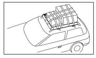
Be sure to securely fix the load with a belt, net, and/or rope. Travelling at high speeds or carrying a load weighing 22 lbs (10 kg) or more results in excessive force being applied to the load due to wind pressure and when starting or stopping the car. Always use a belt.
