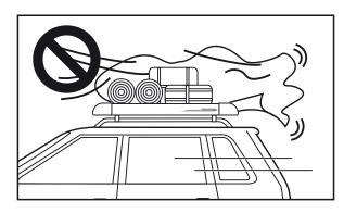
In order to prevent the water proof sheet or similar sheet from flapping, securely fix the sheet, with a belt, net, and/or rope before travelling.
