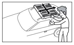
Before loading the cargo and driving the car, be sure to shake the cargo basket to the front, rear, left, right, up and down to check for rattling caused by loose nuts, screws, or bolts and confirm that the cargo basket is securely fixed to the bar.
