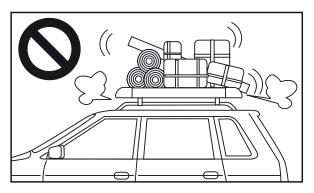
Do not exceed the maximum load capacity when loading. The maximum load capacity differs depending on the combination of the cargo basket and the vehicle model. Refer to the Fit Guide. Refer below for the method on calculating maximum load capacity.
