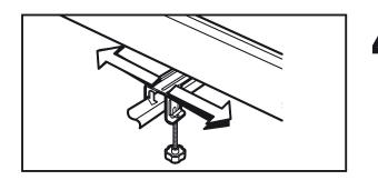
Insert the protruding portion and the screw section into the rail of the side panel so that the mounting hardware faces inside the side panel.
