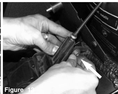
Figure 10 Attach the other vibra mount to the tab on housing. Secure using provided nut and washer. Tighten using 10mm socket and ratchet.
