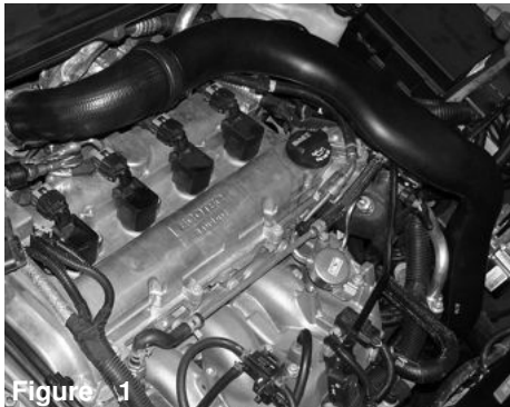
Figure 1 Stock upper intercooler piping to be removed.
