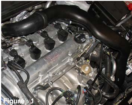
Figure 1 Stock upper intercooler piping to be removed.
