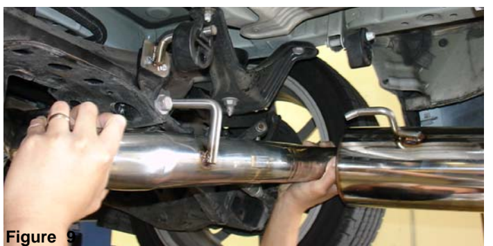
Figure 7 The stock grommet is inserted into the new hanger located on the passenger side rear axle.
