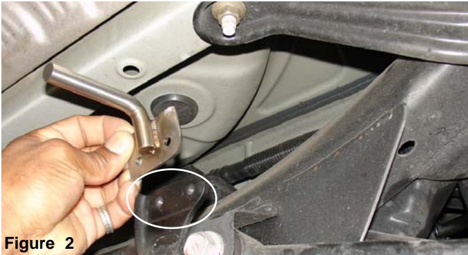
Figure 3 Holes are lined up to the pre-drilled holes on the rear axle brace.
