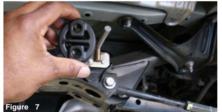
Figure 5 Remove the donut or grommet from the stock hanger located on the driver side rear axle.
