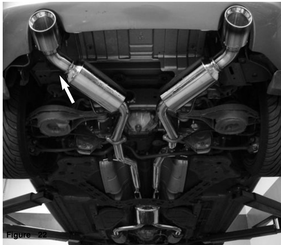
Figure 19 The rear mufflers are now installed. Make your final adjustments for best fitment and then tighten all M10 bolts
