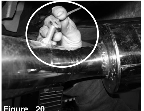
Figure 17 Place a 60mm gasket in between the rear muffler and mid-pipe on both left and right side.
