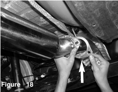
Place a supplied 3.00" gasket inbetween the rear muffler section and the mid-pipe
