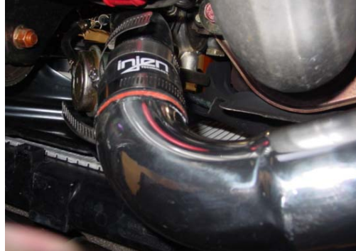
Press the 1.75" straight hose over the turbo inlet, use two .262 Power-bands. Set one end of the hard pipe into the turbo inlet and press the other end into the stock elbow, use two .312 Power-bands on the end tank side.
