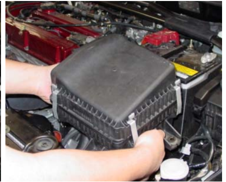
The stock air intake box is removed and the mass air flow sensor is disconnected from the air intake box to be used later in the instruction.
