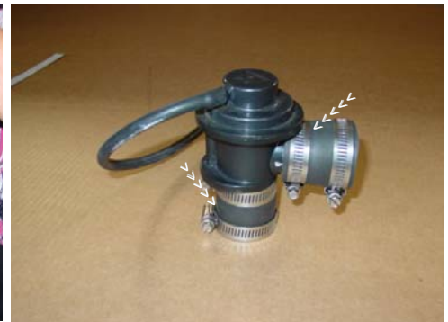
Press the new reinforced short hose over each port on the blow-off valve. Use the .024 mini clamps provided in this kit to secure the hose in place.
