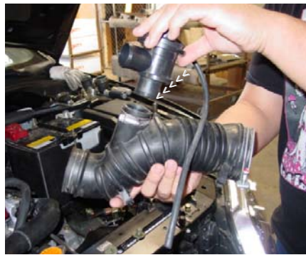
Remove the blow-off valve from the stock intake duct.
