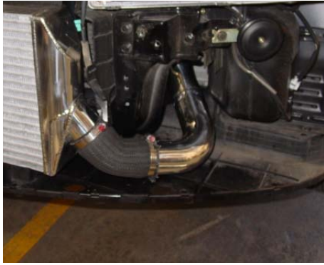
Here is a shot of hardpipe (B) connected to the stock hose on the intercooler tanks. Use two .362 Power-bands to connect hardpipe (B) to intercooler end tank.
