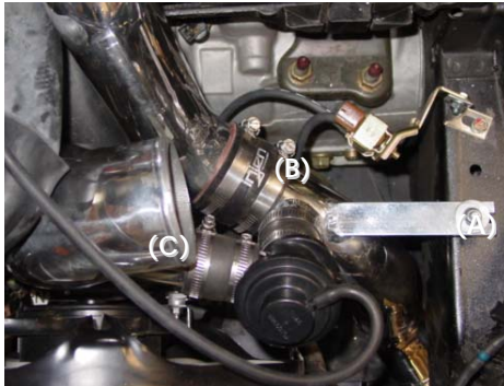
Top view of the bracket (A), blow-off valve (B) and cast intake (C) all connected and ready for the next step.
