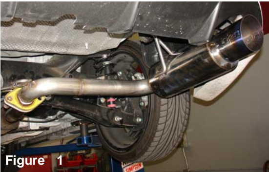
Figure 1 60mm high flowing exhaust system with catalytic converter, titanium tip and test pipe.
