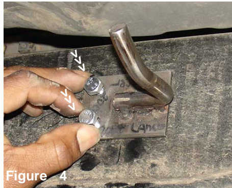
Figure 4 The two m8 bolts in this kit are used to secure the bracket in place.
