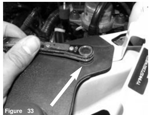
Figure 33 Loosen the 8mm screw above head light.
