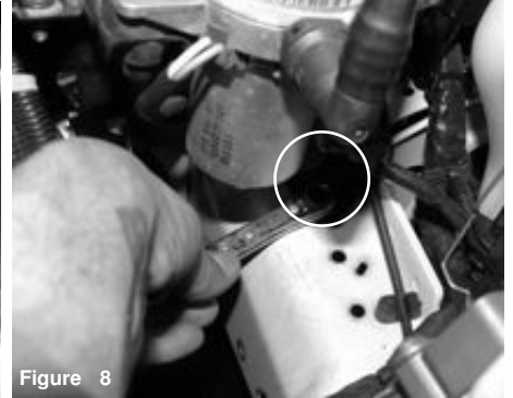
Figure 5 Disconnect the vacuum line from the intake plenum.
