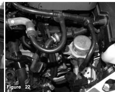
With 10mm wrench, loosen the bolt holding in the stock intake tube bracket.
