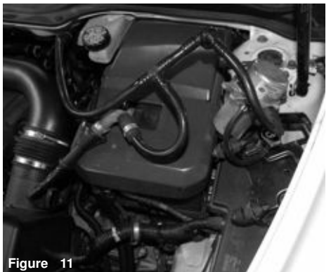
Figure 11 Set aside the complete vacuum assembly on top of battery. This will allow for easier removal of the air box.
