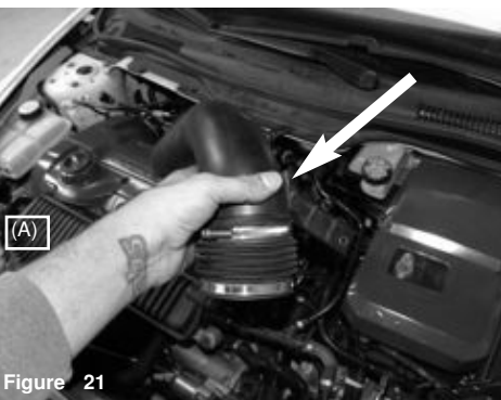
Remove the Complete air box by sliding towards the side of the vehicle. This may require some force. Take caution when removing.
