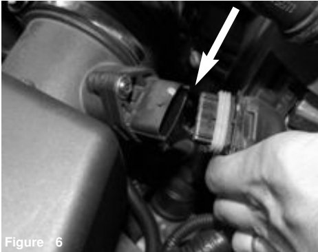
Figure 7 Pull back the factory coupler from air box.
