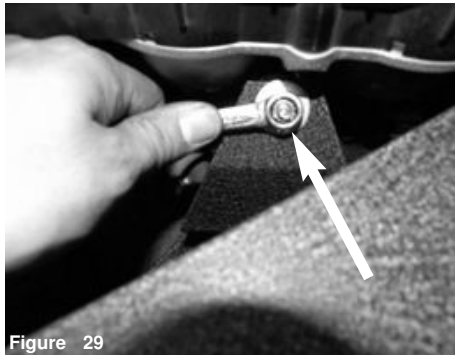
Figure 29 Tighten the stand off stud using provided M6 nut and washer.
