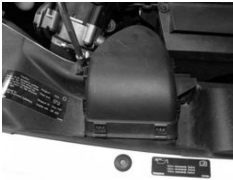
With 8mm socket and ratchet, loosen the 2 bolts holding in the factory scoop.
