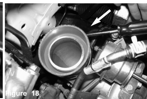
Figure 13 Loosen the screw holding in the factory scoop on the air box. This will be used in the new intake kit.
