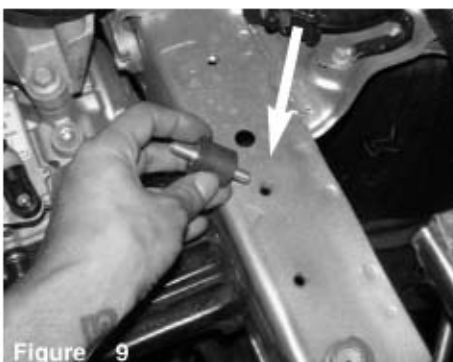
Figure 9 Locate the threaded insert on the frame and install the vibra mount to the insert in photo above.
