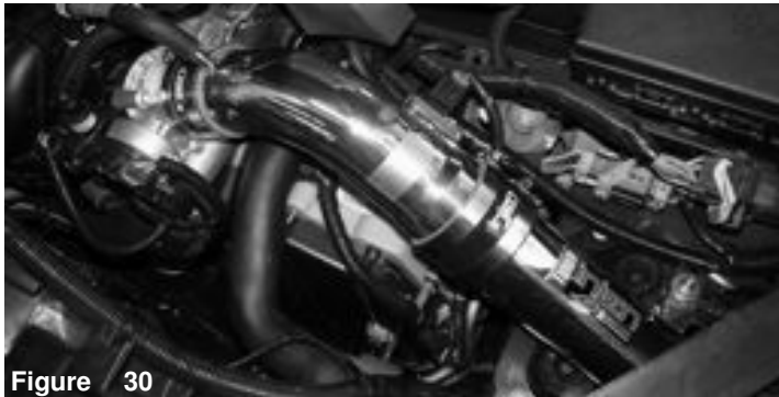
Figure 28 Install the 15mm vacuum line to the engine and to the fitting on the intake tube.
