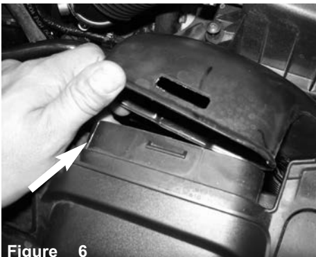
Figure 6 Pull back the ram air scoop from radiator support.
