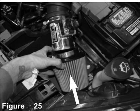
Figure 26 Secure the filter using 8mm nut driver.
