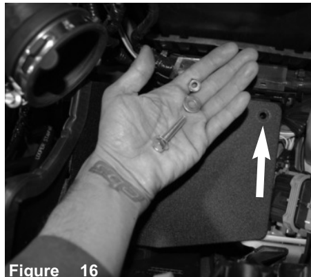
Figure 16 Secure the this hole on heatshield using provided Long M8 bolt, secure back side using washer and M8 locknut.
