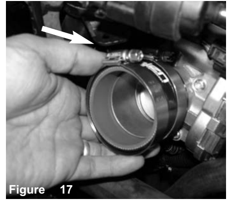
Figure 17 Install the 2-1/4" straight hose with clamps provided to throttle body and tighten on throttle body only.
