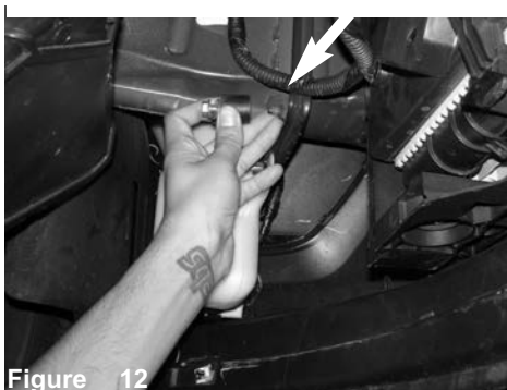
Figure 8 Pull back intake tube from throttle body.
