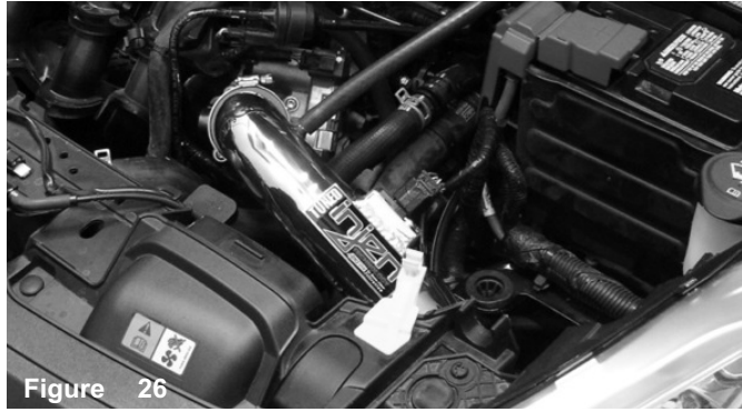
Figure 26 Congratulations! You have just completed the installation of this intake system. Periodically, check the alignment of the intake, normal wear and tear can cause nuts and bolts to come loose. Note: Check clearance and adjust if needed! Failure to check the alignment and adjust the intake can cause damage that will void the warranty. Injen Technology is not responsible for any damages caused by/from improper installation.
