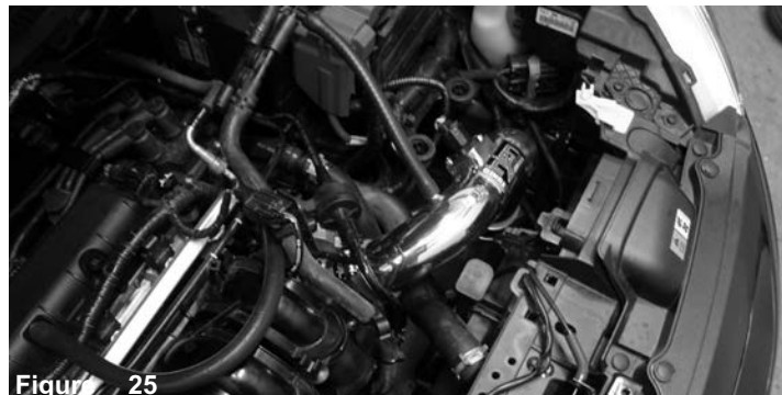
Figure 22 Install provided 10mm hose to crank case on engine side.
