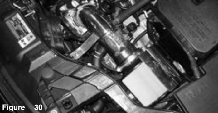
Figure 27 Connect the Vacuum line to the fitting on the intake tube. Note: Make sure it clicks. Re-connect the MAF sensor harness.
