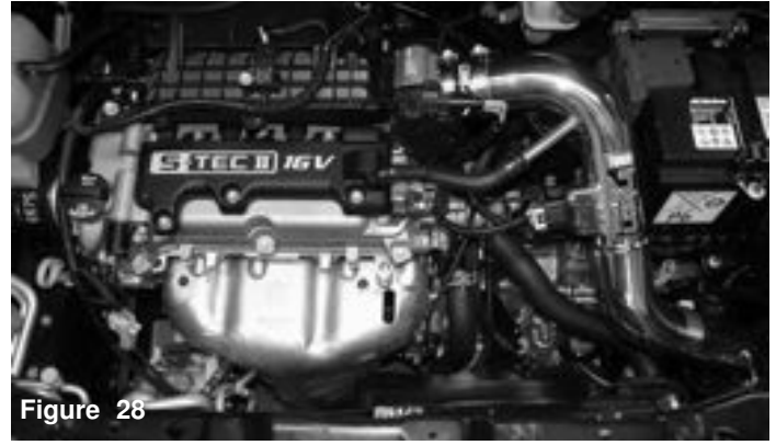
Figure 28 Congratulations! You have just completed the installation of this intake system. Periodically, check the alignment of the intake, normal wear and tear can cause nuts and bolts to come loose. Note: Check clearance and adjust if needed! Failure to check the alignment and adjust the intake can cause damage that will void the warranty. Injen Technology is not responsible for any damages caused by/from improper installation.
