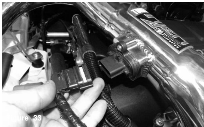
Figure 33 Re-connect the MAF sensor harness. Make sure the intake system is positioned properly and you have clearance.
