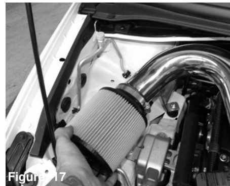
Figure 17 Install the air filter and tighten using 8mm nut driver.
