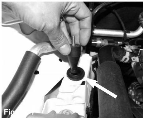
Figure 8 Secure the stand off stud so it seats tightly.
