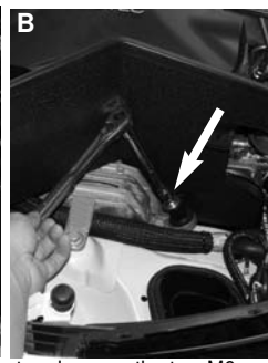
Figure 17 Use a 10mm socket and ratchet and secure the two M6 nuts on the upper left and lower heat shield brackets in figure A and B.
