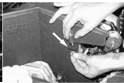
Figure 18 Place the male/male vibramount onto the bracket located on top of the lower heat shield bracket. Use a M6 nut to secure the vibramount to the bracket and then tighten the M6 nut with a 10mm ratchet.
