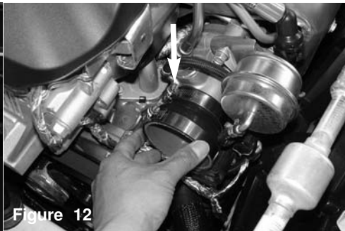
Figure 12 Place the 2.5"x3.0" step hose, #40 and #48 clamp onto the turbo compressor housing inlet. Use a 8mm nut driver and secure the clamp on the turbo side only for now.
