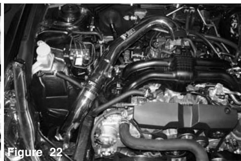
Figure 22 Congratulations! You have just completed the installation of this intake system. Periodically, check the alignment of the intake, normal wear and tear can cause nuts and bolts to come loose. Failure to check the alignment and adjust the intake can cause damage that will void the warranty.
