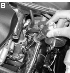
Figure 16 Mount the lower heat shield bracket onto the stand off stud from figure 10. Then place a washer and a M6 nut onto the stand off.
