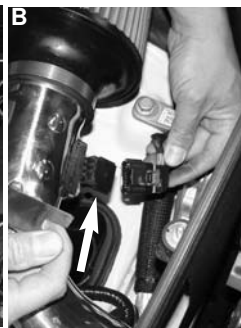
Figure 20 Figure A: Position the intake pipe through the heat shield opening. Figure B: Run the MAF sensor harness under the heat shield and then connect the harness to the MAF sensor.
