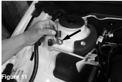
Figure 11 Place the M6 male/female vibramount onto the right threaded stud located on the passenger side shock tower. (The stud without the factory nut)
