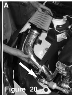
Figure 20 Figure A: Position the intake pipe through the heat shield opening. Figure B: Run the MAF sensor harness under the heat shield and then connect the harness to the MAF sensor.
