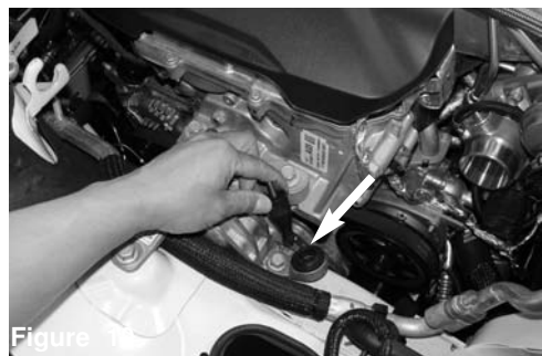
Figure 6 Once the clamp is loose, pull the turbo duct off the turbo compressor housing inlet.
