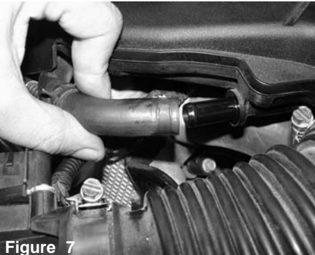
Figure 7 With pliers pull back crank case line.
