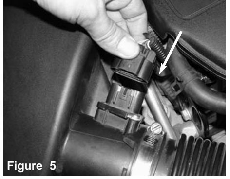
Figure 5 Disconnect the MAF sensor harness.
