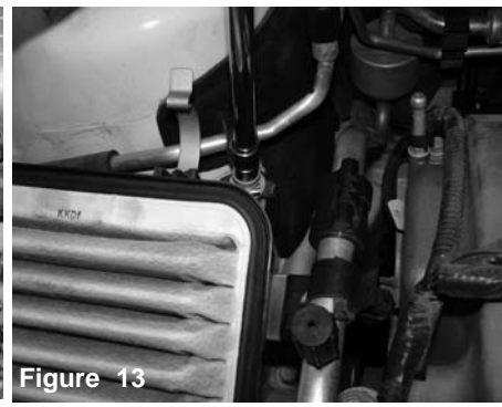
Figure 13 With 10mm socket and ratchet, loosen and remove the bolt holding in A/C line and air box.
