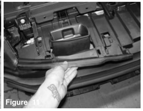
Figure 8 Pull back the second grommet on the back of the air box.
