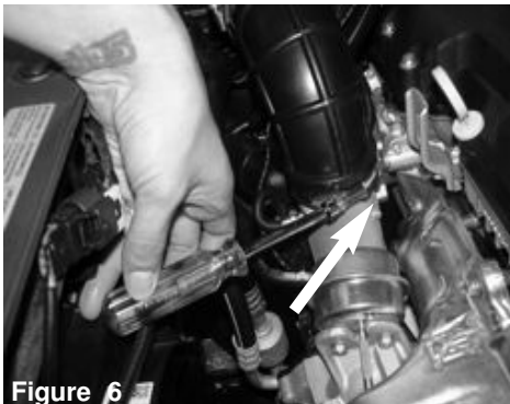
Figure 6 Loosen the clamp on the turbo using 7mm nut driver.
