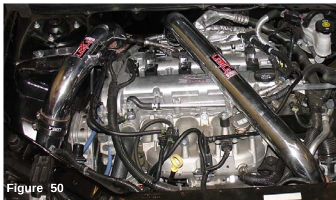
Figure 50 Periodically, check the fitment of both intake systems. Normal driving conditions may loosen nuts, bolts and clamps causing intakes to shift resulting in damage to automotive parts.
