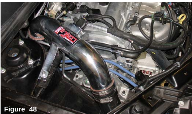
Figure 48 Check the connection of the intake bracket to the vibra-mount and the alignment of the primary and secondary intakes. Everything should be properly aligned to prevent damage to the cold air intake.
