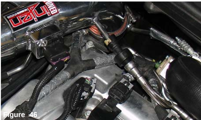
Figure 46 Check the harness clip and vacuum lines for proper fitment. Make sure there is good contact between the harness clip and mass air flow sensor, check for any possible vacuum leaks in the vacuum connections.
