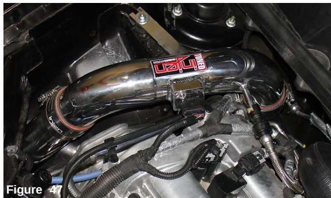
Figure 47 Periodically, check the fitment of both intake systems. Normal driving conditions may loosen nuts, bolts and clamps causing intakes to shift resulting in damage to automotive parts.
