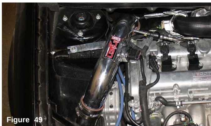
Figure 49 Congratulations! You have just completed the installation of the best air intake system made. Prior to driving, start the engine, and listen for any air leaks, rattling or vibration. Allow 5 to 10 minutes for the ECU to adjust to the added volume or air created by the cold air intake.
