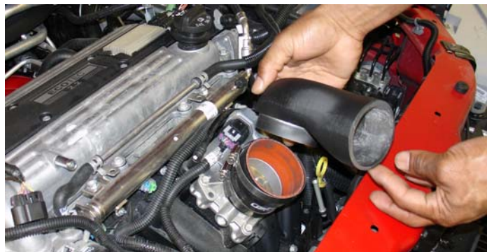
Take the specially designed aluminum elbow and press it over the throttle body hose.
