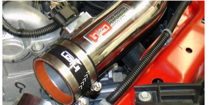
To convert your intake system into a cold air intake take the 3" straight hose and press it over the end of the primary intake. Use two clamps from the kit to place them over the hose and tighten the clamp on the intake.
