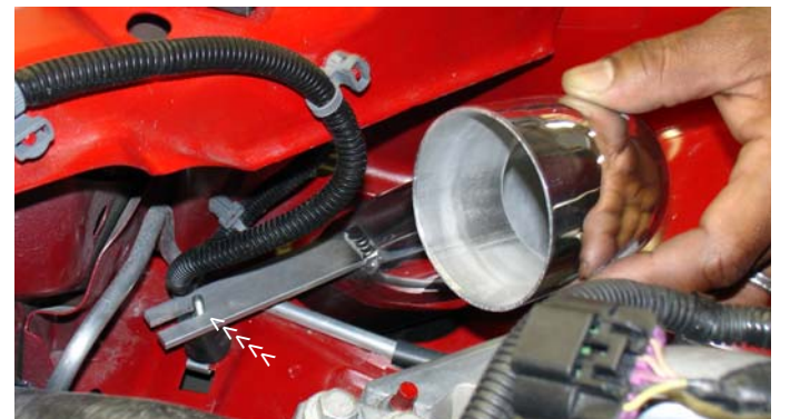
Once the secondary intake has been inserted into the resonator opening align the bracket to the vibra-mount stud.
