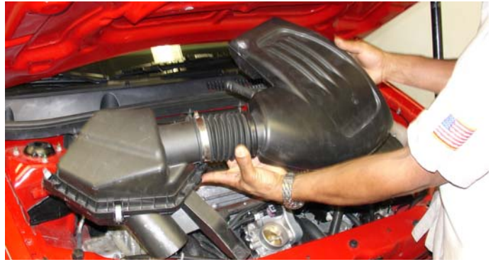
Once the stock clamps have been loosened remove the entire air intake box from the engine compartment.
