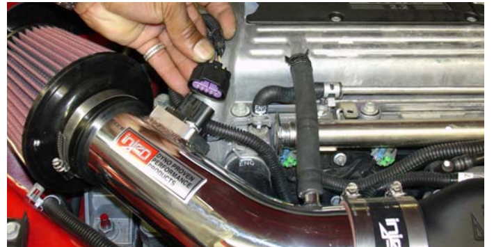
Locate the stock harness clip and plug it into the MAFS. Press the harness into the sensor until you here it snap in place.
