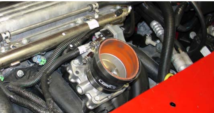
Press the 2 3/4" x 3" step hose over the throttle body and use two clamps on the hose, tighten the clamp on the throttle body at this time.
