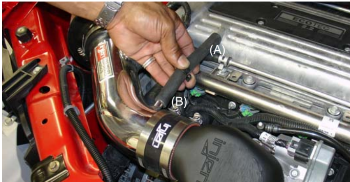
Take the 7" 12mm heat hose and press one end over the crankcase port (A) and the other end over the intake port (B).
