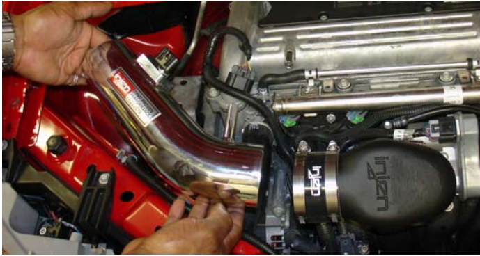
Take the primary intake and press the end into the hose on the cast aluminum elbow.
