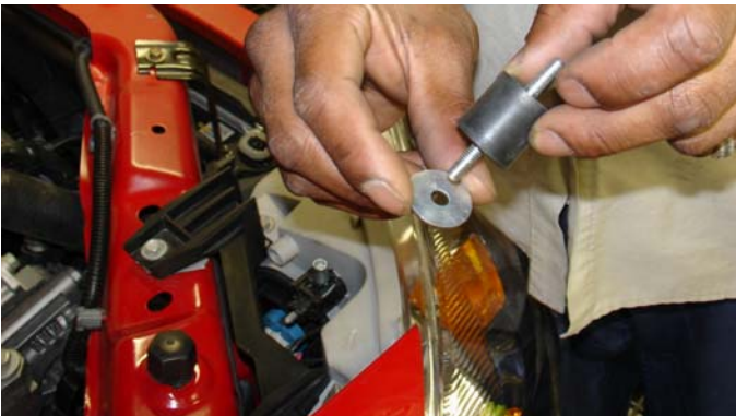
Take the fender washer and place it over the vibra-mount stud. This fender washer will be used as a spacer to raise the primary intake.
