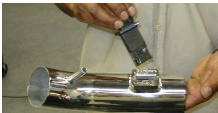
Take the MAFS removed earlier from the stock air intake box and press it into the machined adapter. Use the stock sensor screws to reattached the MAFS into the machined adapter.
