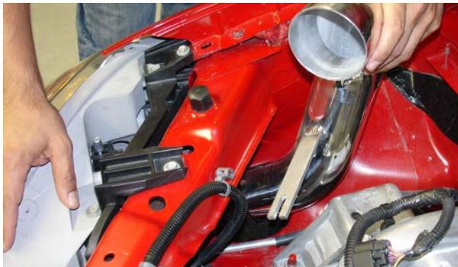
Take t the secondary intake and insert it into the resonator opening.
