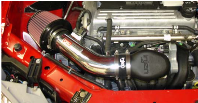
The short ram is now fully installed and ready to go.
