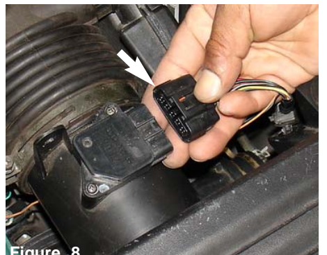
Figure 8 Disconnect the electrical sensor harness from the mass air flow sensor.
