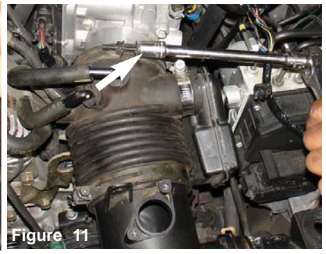
Figure 8 Disconnect the electrical sensor harness from the mass air flow sensor.
