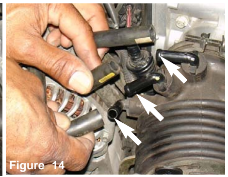
Figure 13 All three vacuum lines are disconnected from the air intake duct connected to the throttle body.
