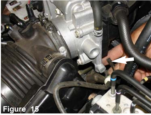
Figure 16 Disconnect the vacuum line as shown above.
