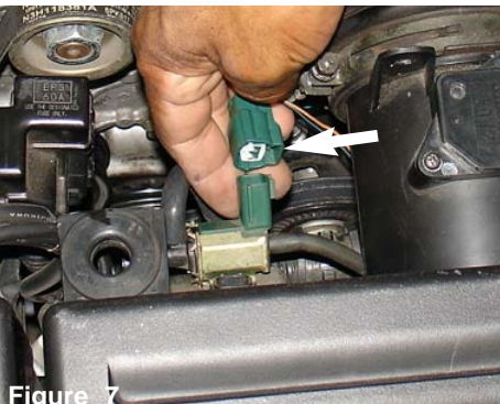
Figure 7 Depress the tab on the green electrical clip and pull the clip from the vacuum switching valve.
