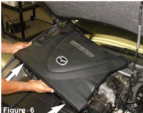
Figure 6 pull up on the stand offs located in front of the engine cover. A slight tug up will be required to pull the stand offs out of the stock grommet.
