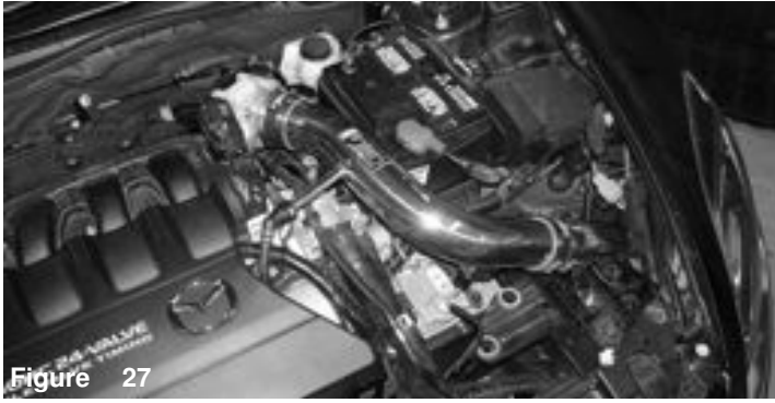
Figure 27 If vehicle was jacked up, lower vehicle. Connect battery terminals. For short ram install, remove the lower intake assembly and place filter on upper intake tube assembly. See figure 28.
