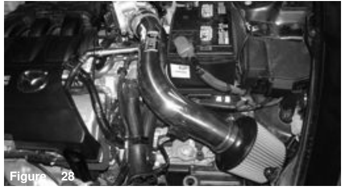
Figure 28 Align the entire intake for the best possible fit. Once you have rechecked and cleared the intake from all moving parts, continue to tighten all nuts, bolts and clamps.
