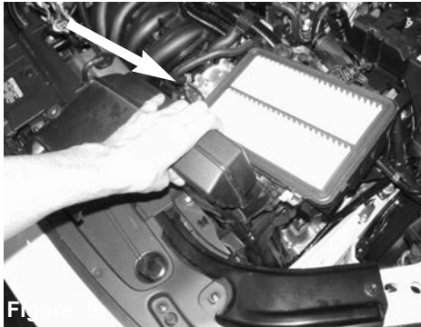
Figure 9 Now lift up and remove the bottom half of the air box.
