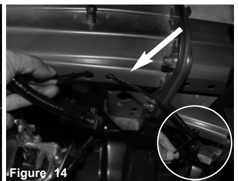
Figure 11 Pull back the harness from the bracket, remove the bracket from the vehicle.
