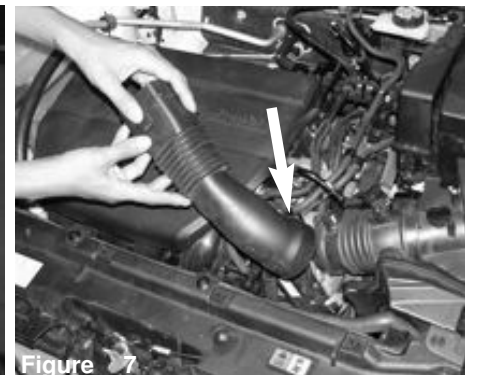
Figure 7 Carefully remove the plastic air intake duct.
