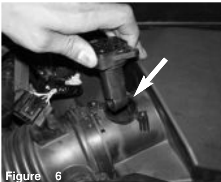
Figure 6 Carefully remove the electrical MAF sensor from sensor housing.
