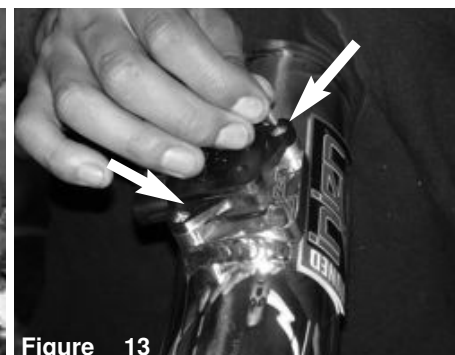
Figure 13 Insert the electrical MAF sensor to intake tube. Secure the sensor by using the provided M4 button head screws.
