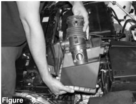
Figure 8 Remove the entire air intake box assembly from the engine compartment.
