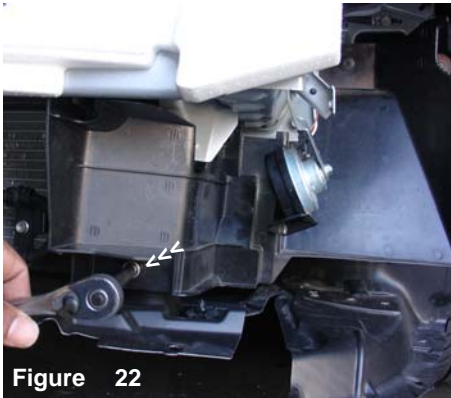
Figure 22 The second m6 bolt is removed from the splash guard.
