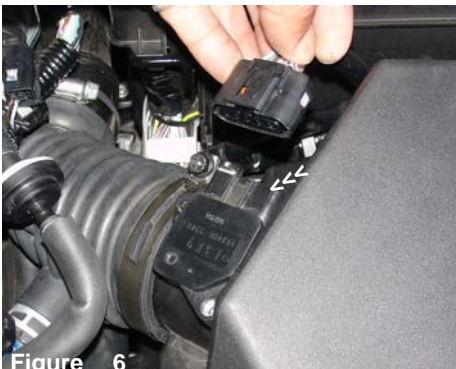
Figure 6 Remove the electrical harness clip from the air mass sensor as shown above.
