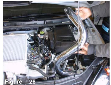
Figure 26 Lower the cold air intake into the engine compartment and into the bumper area.
