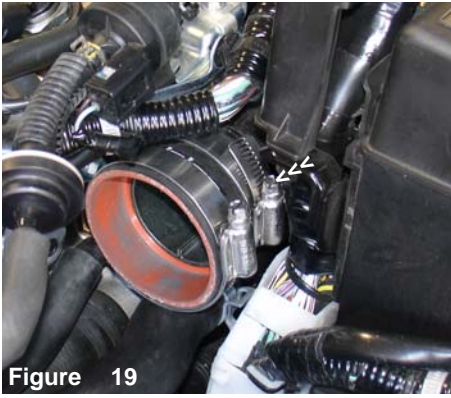
Figure 19 Press the step hose over the turbo inlet. Tighten the power-band on the turbo inlet side for now.
