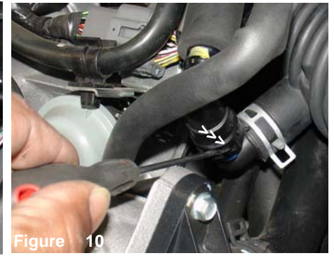
Figure 9 Loosen the clamp that connects the air duct to the turbo inlet.
