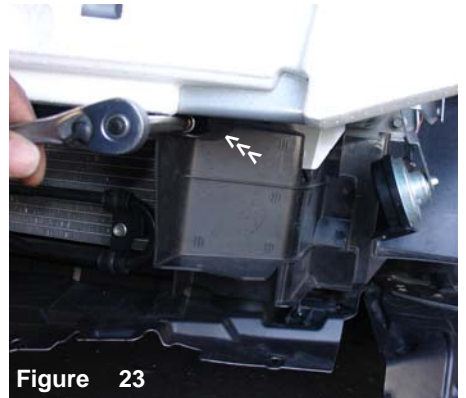
Figure 23 The third and final m6 bolt is removed from the splash guard.
