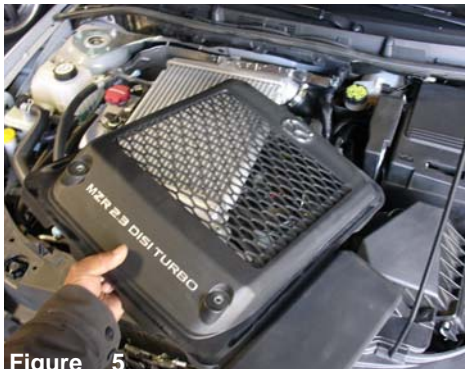
Figure 5 The intercooler cover is now removed
