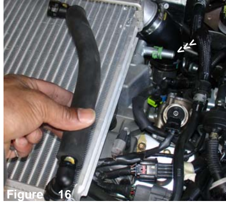
Figure 16 The upper breather hose is disconnected from the breather port as shown above. The stock hose is no longer used in this installation.
