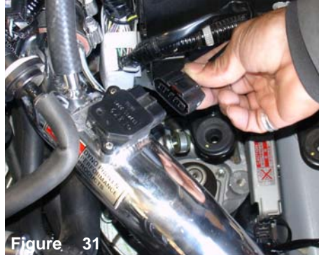
Figure 31 Press the electrical harness clip to the air mass sensor until it snaps in place.
