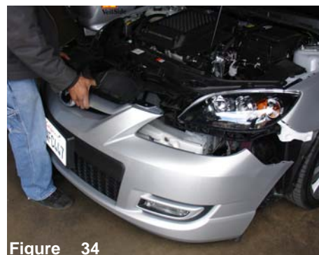
Figure 34 Once you have aligned and tightened all nuts, bolts and clamps, continue to install the front bumper to its original position.
