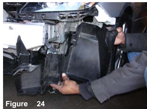
Figure 24 Once all bolts have been removed, continue to pull the splash guard out of the bumper section.
