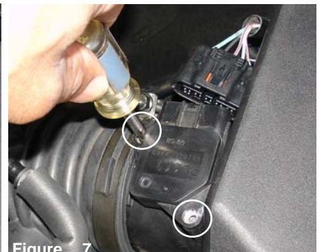
Figure 7 Remove the two screws that fastens the air mass sensor to the sensor housing.
