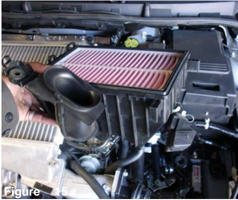
Figure 15 The lower air box cleaner is now pull out of the rubber plungers
