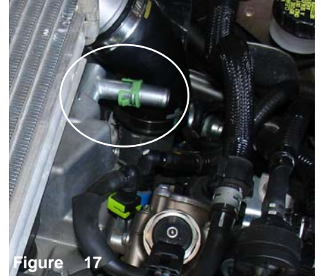
Figure 17 The green locking tab is also removed from the vacuum port.
