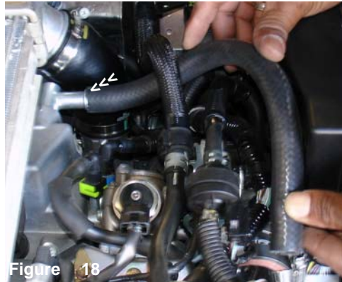
Figure 18 Press the 14"- 15mm breather hose over the vacuum port as shown above.
