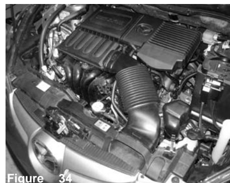
Figure 33 Re-install the ECU cover.
