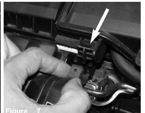
Figure 7 Un-clip the upper half of airbox/engine cover.
