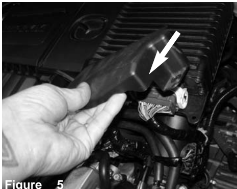
Figure 5 Loosen the clips holding in the Harness cover and remove.
