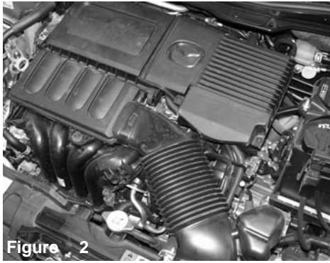
Figure 3 Remove the factory scoop from vehicle.
