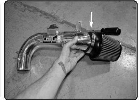
**15.** Now install the air filter to the tube and tighten using 8mm nut driver.
