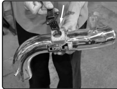
**13.** Install the MAF sensor into the new intake tube.
