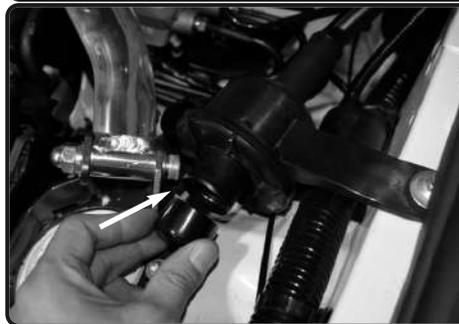
**22.** Install the provided vinyl cap to the sound tube muffler.
