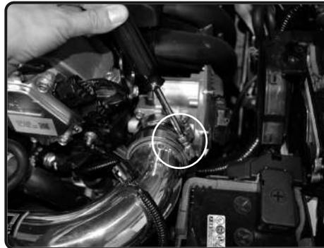
**18.** Position for the best fit and tighten the clamp on throttle body.
