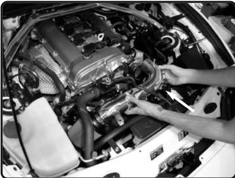
**16.** Install the 2.75" straight hose with clamps to throttle body. Now install intake tube assembly and position the tube to straight hose.
