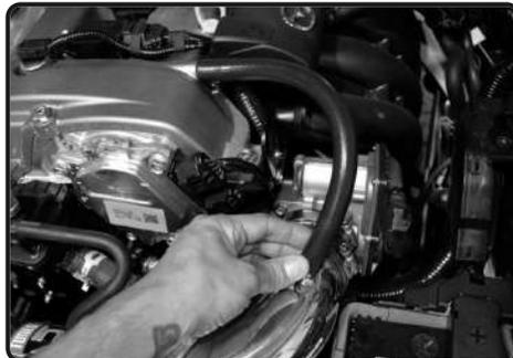
**21.** Now connect the provided 10mm hose to the engine fitting and intake tube.
