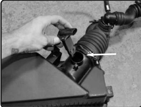
**12.** Loosen and remove the MAF sensor from the factory air box.
