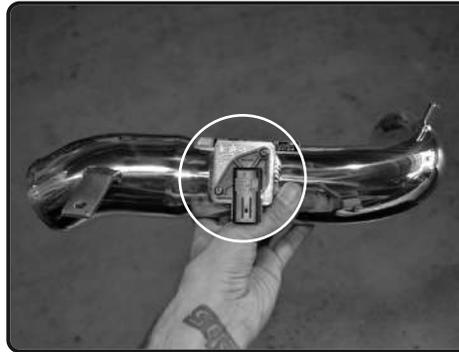
**14.** Secure using M4 button head screws and tighten using 2.5mm allen key.
