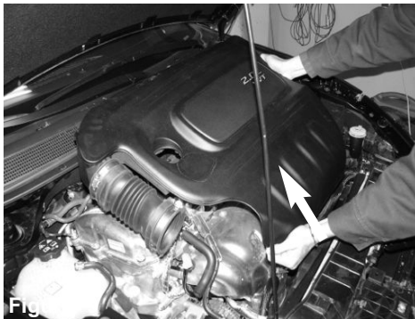
Figure 6 A) Loosen the clamp on the throttle body. B) Loosen and remove the
