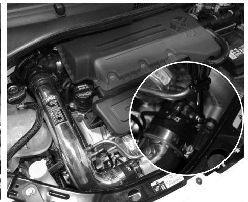
Install the step hose to the turbo with clamps. Tighten the clamp on turbo only. Install new intake tube and position intake tube to factory 90 elbow and turbo. Position best fit and tighten. Re-connect vacuum line and secure. Congratulations! You have just completed the installation of this intake system. Periodically, check the alignment of the intake, normal wear and tear can cause nuts and bolts to come loose. Note: Check clearance and adjust if needed! Failure to check the alignment and adjust the intake can cause damage that will void the warranty. Injen Technology is not responsible for any damages caused by/from improper installation.
