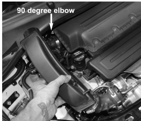
Loosen clamp on turbo. Loosen clamp on the 90 elbow. Disconnect the vacuum line using pliers. Remove the factory intake tube.
