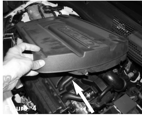
Figure 5 Pull out the crank case line from the air box.
