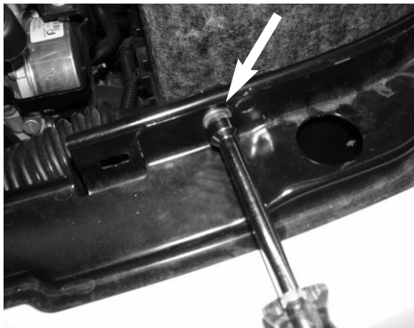
Figure 6 With 8mm socket or nut driver, loosen the bolt holding in the 90 degree plastic snorkel.
