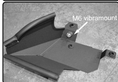
10. Install the M6 vibramount to the threaded insert on the heatshield and secure.
