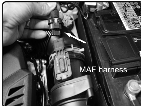
7. Disconnect the MAF sensor harness from the intake system.
