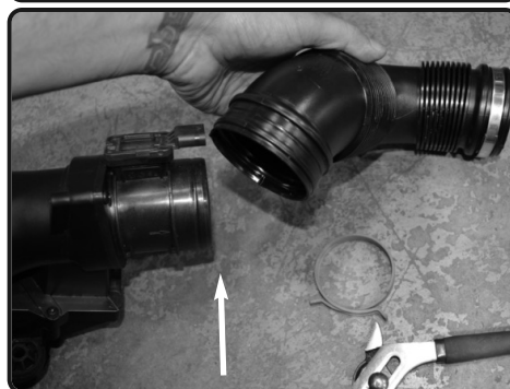
6. Un-clip and remove the intake tube from the MAF sensor.
