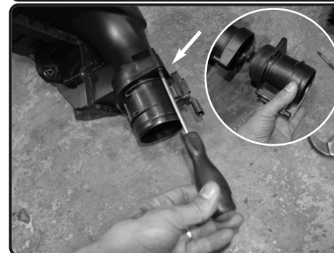
7. With T25 torx bit, loosen the 1 bolt holding in the MAF sensor. Rotate and remove the MAF sensor from the air box. Save for later install.
