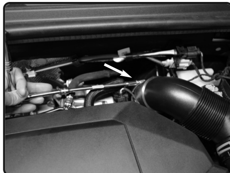
2. Loosen the clamp on the turbo using 7mm nut driver.
