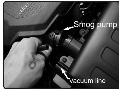
3. Disconnect the smog pump line and the vacuum line from the intake system.
